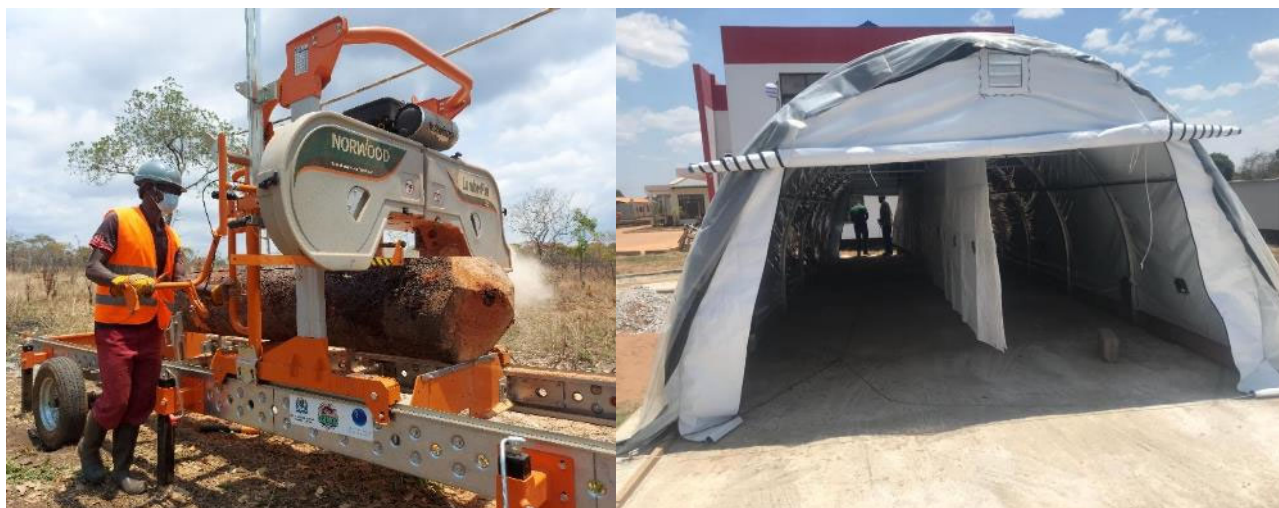
Figure 2. The solar timber drying kiln and portable sawmill owned by communities.
