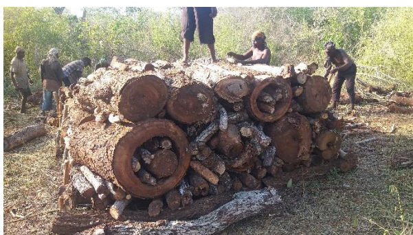
Plate 11: Charcoal making group establishing a charcoal kiln at Kwedikabu Village, Handeni District, Tanga Region.
