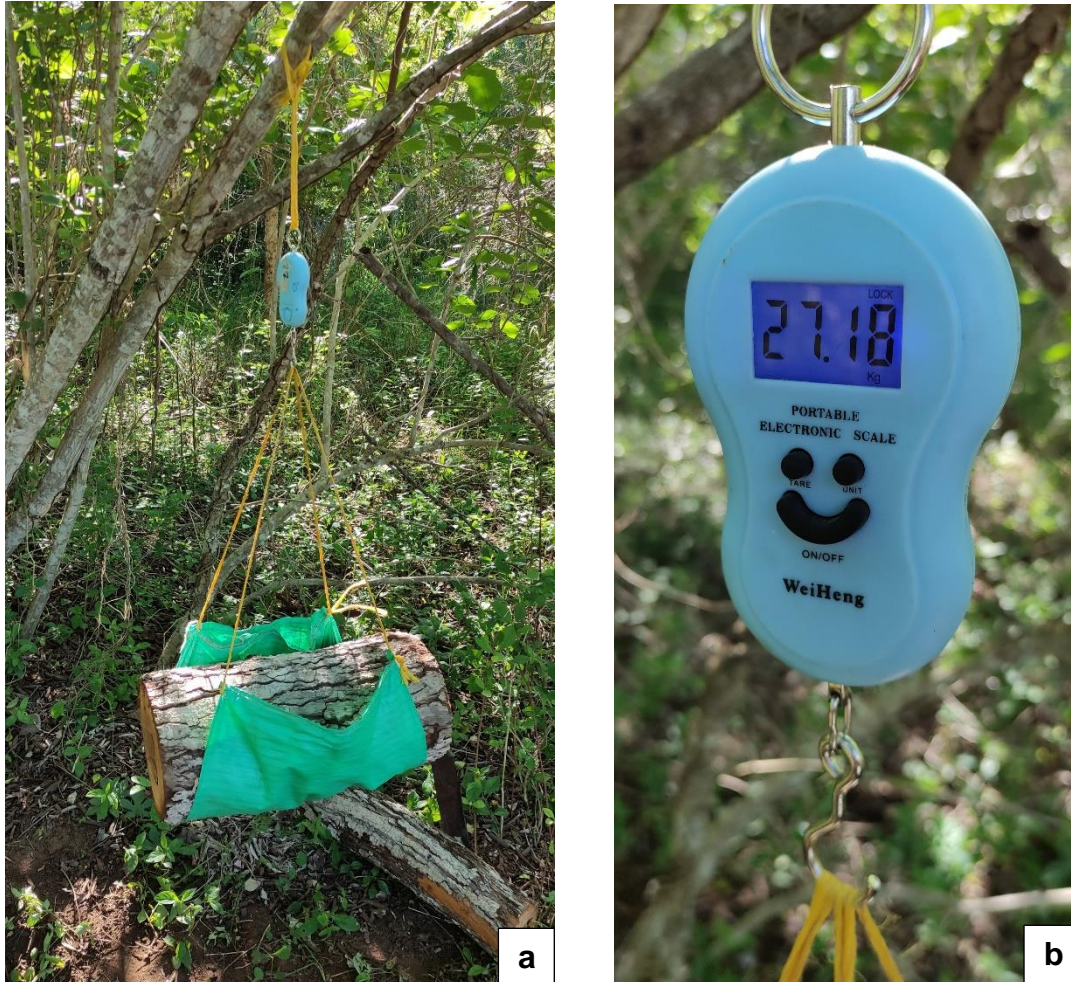
Plate 2: A billet being measured for weight (a) using portable electronic hanging scale (b)
