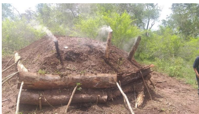
Plate 14: Charcoal making group establishing a charcoal kiln at Kwedikabu Village, Handeni District, Tanga Region.
