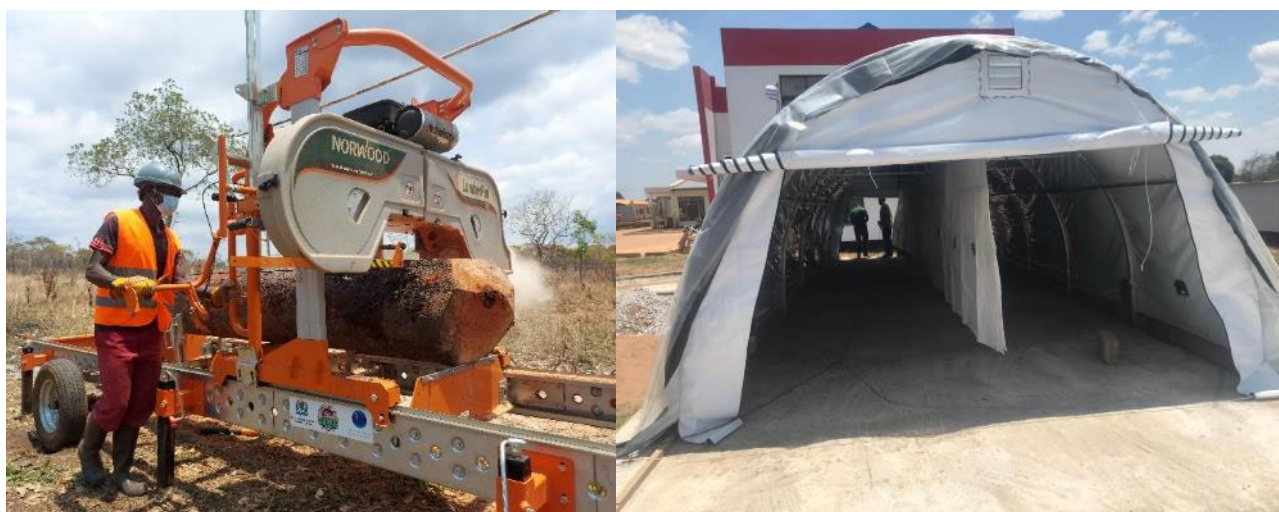
Figure 3. The solar timber drying kiln and portable sawmill owned by communities.
